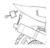
installation pitch angle the radar surface dips  $10\pm2^{\circ}$  Note: the outlet is at the top
