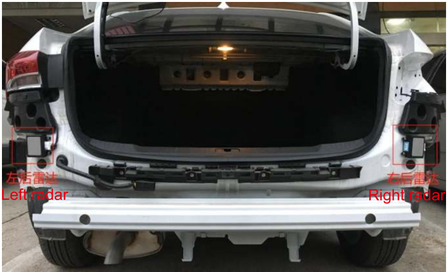
Physical Diagram for Installation Position of Radar
